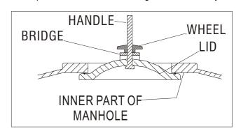
Introduce the lid in the manhole, leaving it leveled and centered. The lid must be supported by the handle, as this will avoid that it could fall into the tank and damage any of its parts.
