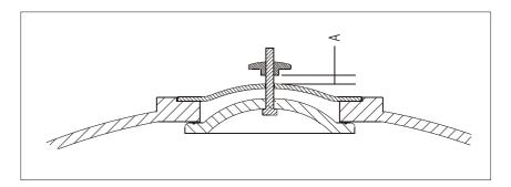
Once the filter has been completely filled with water, start the performance of installation, venting manually to eliminate all the air that could be inside the filter, as the presence of air impairs the filter performance.
