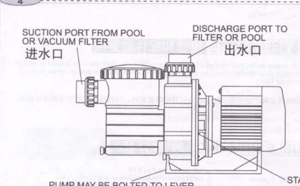
PUMP MAY BE BOLTED TO LEVER FOUNDATION OR MOUNTING BRACKET
